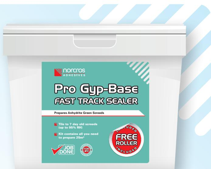
Norcros Pro Gyp-Base is a 3-part preparation system which allows ceramic & porcelain tiles to be fixed onto anhydrite screeds that are a minimum of 7 days old (95% Relative Humidity). The system offers a fast track solution when tiling onto anhydrite screeds, greatly reducing the minimum drying times generally quoted for this type of screed of 1mm/day up to 40mm and an additional 1mm/2 days above 40mm thickness.
